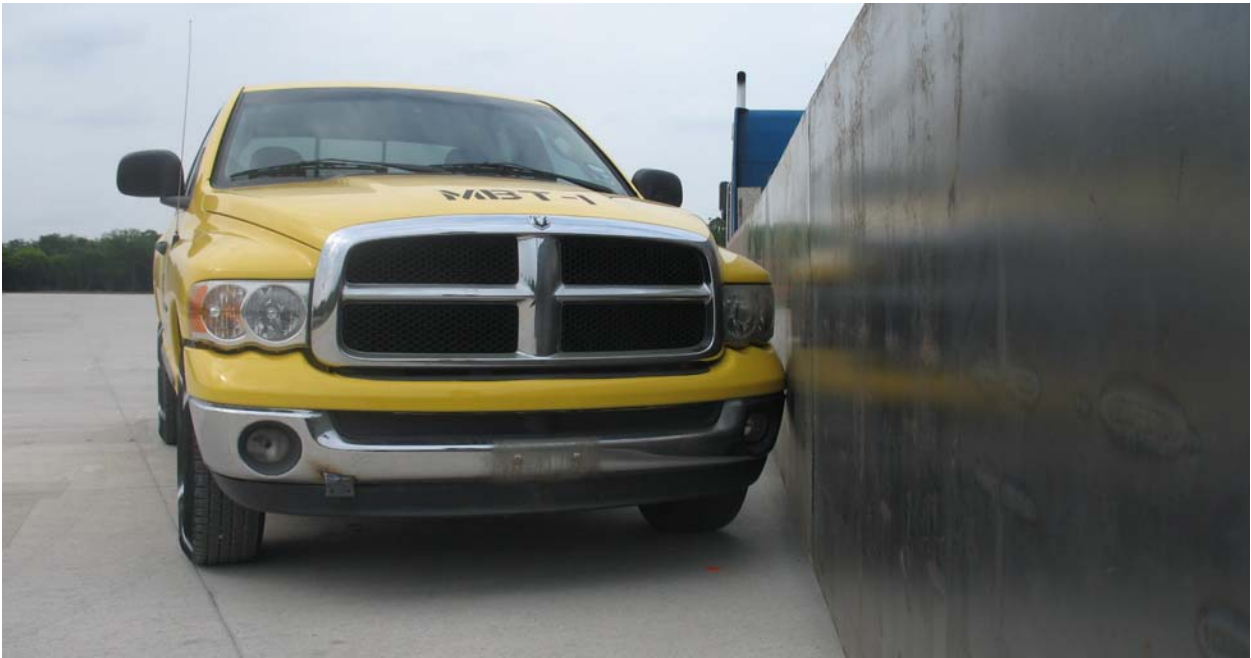
Figure 2.10 – Test Vehicle Bumper Height
