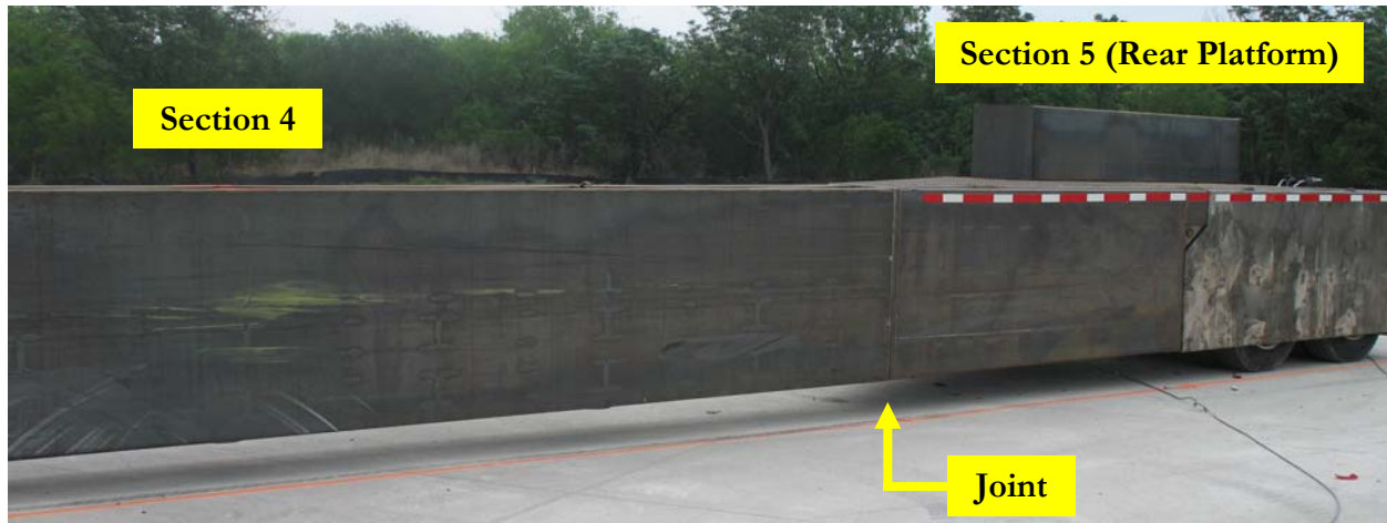
Figure 3.7 –Mobile Barrier Trailer after the Crash Test (Joint Connecting Sections 4 and 5)
