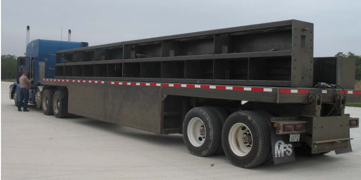
Figure 2.3 – Mobile Barrier Trailer – Disassembled with Wall Panels Removed for High Speed Transport
