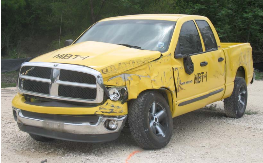
Figure 3.13 – Damaged Test Vehicle (Left Side)
