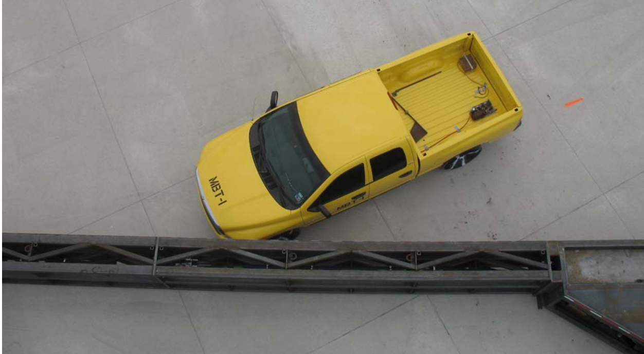
Figure 2.11 – Overhead View of Test Vehicle Impact Angle
