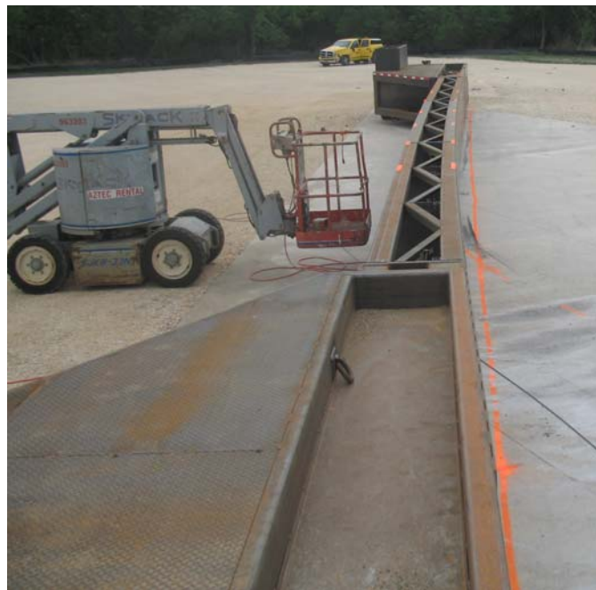
Figure 3.8 – Overhead View of Mobile Barrier Trailer after the Crash Test
