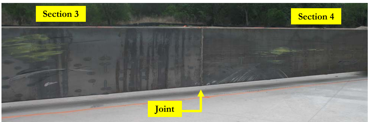
Figure 3.6 – Mobile Barrier Trailer after the Crash Test (Joint Connecting Sections 3 and 4)
